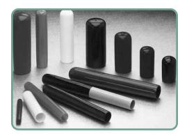
Long Caps come in diameters ranging from 3/16" through 3-1/2". Most sizes are available in inside lengths up to 5-1/4", in 1/16" increments and many are available to 8" lengths. Excellent as pipe protectors, grips, caps for boiler tubes, connectors and cable end seals. Tough and durable, Long Caps are also used in many masking applications.
