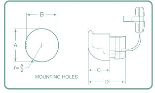
Provides the same protection for your power supply cable as the straight-thru type and exits the cable flush against the chassis, saving space and directing the cable parallel to the panel.
