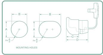
Provides the same protection for your power supply cable as the straight-thru type and exits the cable flush against the chassis, saving space and directing the cable parallel to the panel.
